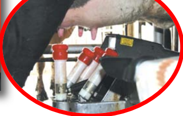
To ensure optimal pre-treatment the utter and each teat is brushed with the mechanical brush system not just water. This process begins right after the cows enter the cow box.
