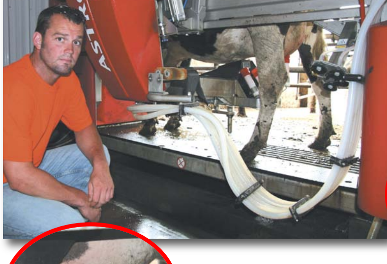
To ensure optimal pre-treatment the utter and each teat is brushed with the mechanical brush system not just water. This process begins right after the cows enter the cow box.
